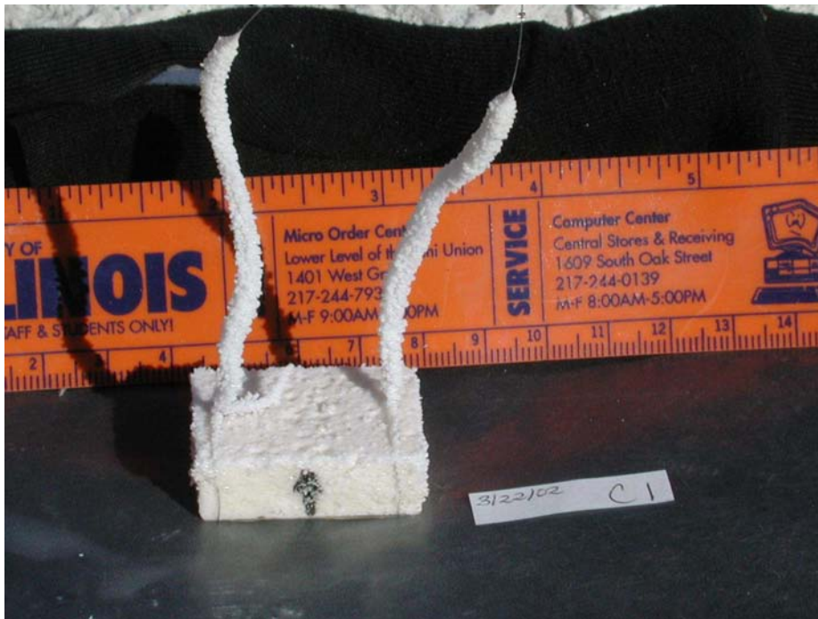
Figure 5.5: Travertine block left in the hot spring for 24 hours. Notice the large amount of deposition on top of the travertine and on the wires. This high deposition creates a very hostile environment for microbial life, which must somehow avoid being encrusted (fig. 5.6). Picture courtesy of George Bonheyo and Bruce Fouke.
