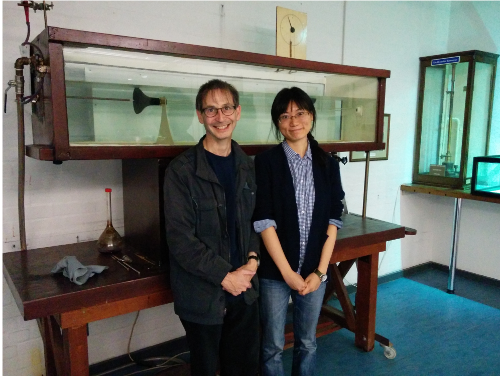
Figure 10.22: Reynolds' original apparatus on the display in Manchester University.
