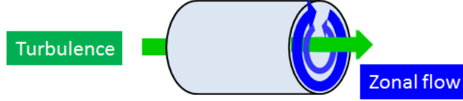
Figure 10.2: Sketch of the zonal flow and turbulent fluctuations. The zonal flow (green) is the composition of layers of the azimuthal flows with alternating directions that change with time as well as their magnitude. The turbulence mode is the remaining part with smaller scales of fluctuations whose overall propagation is longitudinal.
