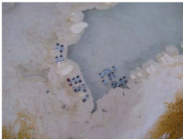
Figure 7.3: Photograph showing washers placed in the hot spring to measure precipitation. The color coded electrical tape denotes how long the washers were left in the spring (either 4, 12, or 48 hours).
