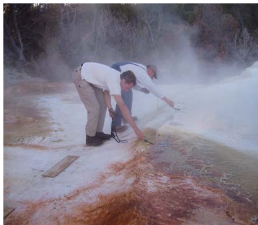
Figure 7.4: Photograph showing collection of pH, temperature, and TDS data near the washers located at sample location 2.4.5. John Veysey and Tom Schickel are shown for scale. They stood on boards to protect carbonate features.
