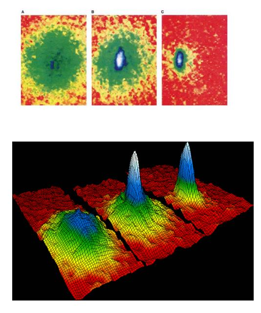
The temperature of the three plots are 400 nK, 200 nK and 50 nK (from left to right), respectively. The field of view of each image is 200 microns by 270 microns. Observation was made with laser pulse resonant with the  $5S_{1/2}$ , F=2 to  $5P_{3/2}$ , F=3 transition.
