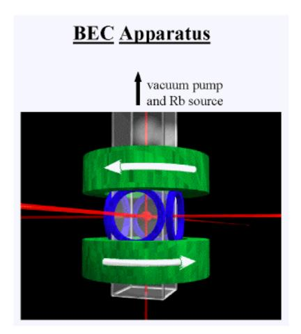
In this experiment, six laser beams intersect in a glass cell, creating a magneto-optical trap (MOT). Rb-87 atomic gases is contained in the cell which is 2.5 cm square by 12 cm long, and the beams are 1.5 cm in diameter. The coils generating the fixed quadrupole magnetic field and rotating transverse components of the TOP trap magnetic fields are shown in green and blue, respectively.
