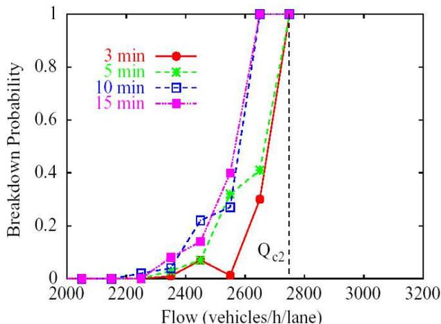
FIG. 3: Probability of free-traffic breakdown as a function of traffic flow. Several waiting times are shown, showing the instability of free-traffic flow at high-flow rates [10].
