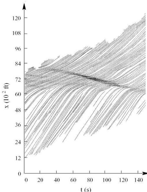
FIG. 5: Data for a “phantom traffic jam,” taken using aerial photography. Broken lines indicate lane changes. As the line slopes (vehicle velocities) decrease, the line density (spatial vehicle density) increases, corresponding to spontaneous traffic jam. The jam front then propagates upstream with constant velocity [7, 17].
