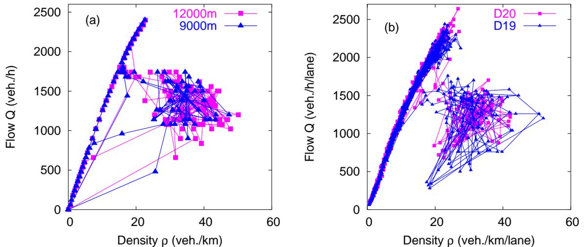
FIG. 7: Graphs of traffic flow as a function of traffic density. Here we compare simulated data for an intelligent-driver model that incorporates short-term driver memory (a) to empirical data taken on the German freeway A9-South near Frankfurt on July 31, 2001 (b). There is excellent agreement between theory and experiment, showing the characteristic free and congested regimes in addition to hysteretic effects. Figures and data from [19].
