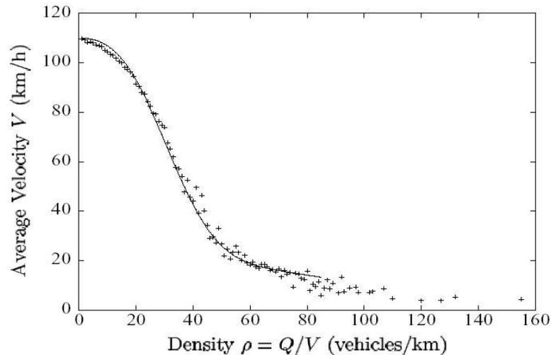
FIG. 1: Comparison of empirical velocity-density relations for different definitions of the average velocity. The ‘plus’ symbols represent one-minute averages determined using the harmonic velocity formula:  $V = \frac{1}{\langle 1/v_\alpha \rangle}$ . The solid line is a fit to the same data interpreted using the traditional arithmetic formula,  $V = \langle v_\alpha \rangle$  [9].
