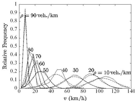
FIG. 4: Empirical velocity distributions for vehicle densities ranging from 10 to 90 vehicles per kilometer. The solid lines represent data while the dashed lines are normal distributions having the same mean and standard deviation [9, 12].
