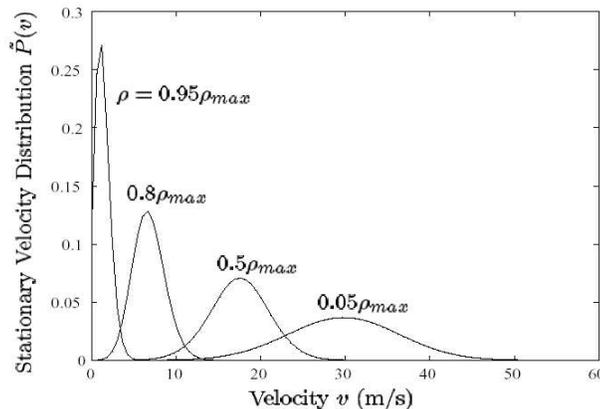
FIG. 8: Velocity distributions shown for different fractions of maximum vehicle density. These distributions were obtained through numerical solution of the gas-kinetic traffic model [20].
