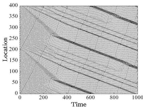
FIG. 6: Simulated trajectories calculated using the optimal velocity model [18] for every fifth vehicle. As shown, this model is able to reproduce the phenomenon of “phantom traffic jams”, shown experimentally in figure 5 [9].
