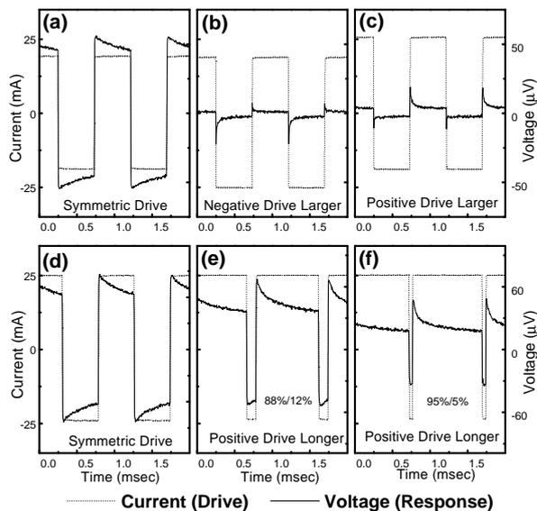
FIG. 4 Effect of changing the symmetry of the driving current. (a),(d) symmetric bidirectional pulses; (b),(c) drive amplitude asymmetry; (e),(f) temporal asymmetry.
