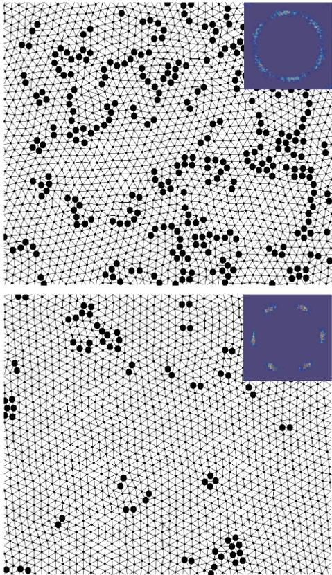
FIG. 6 Delaunay triangulation and structure factor,  $S(\mathbf{k})$  for steady forces (up) and oscillatory square-forces (down). The more-ordered vortex configuration at the down panel was obtained after 500 cycles of the oscillatory force applied to the disordered state in the up panel. See text.  $F^L = 0.0118f_0$  (in the horizontal direction).
