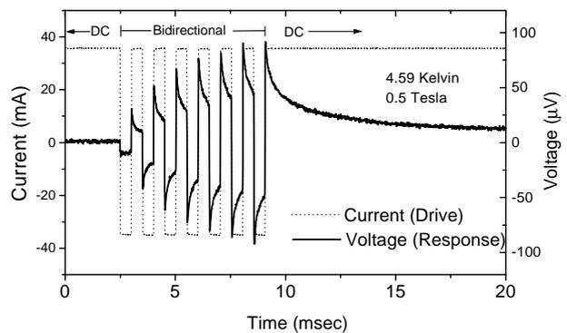
FIG. 5 In this measurement a dc current was first applied for several seconds. Then several bidirectional pulses were applied after which the current was set back to dc.
