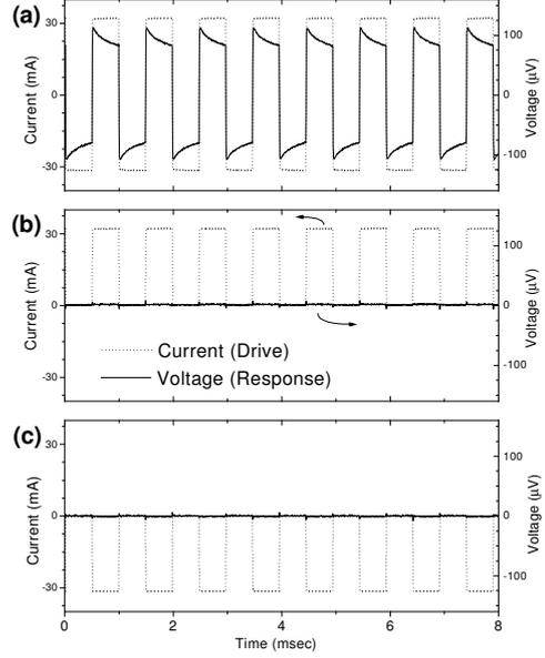
FIG. 3 The response of the flux lattice at  $H=0.5$  T and  $T=4.59$  K to bidirectional pulses (a), positive unidirectional pulses (b), and negative unidirectional pulses (c).
