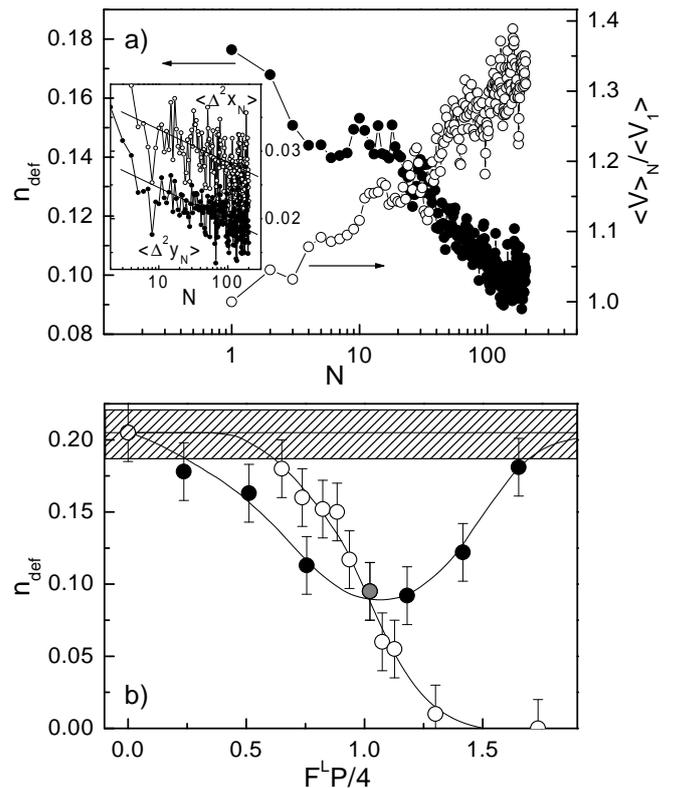
FIG. 7 Dynamical ordering. (a) Defect concentration,  $n_{def}$ , average absolute-velocity,  $\langle v \rangle$ , and average quadratic displacements of vortices per cycle,  $\langle \Delta^2 x_N \rangle$  and  $\langle \Delta^2 y_N \rangle$  vs. the number of cycles,  $N$ . (b)  $n_{def}$  as a function of  $F^L P/4$  after 100 cycles (filled circles:  $F^L$  fixed, open circles:  $P$  fixed). The point  $F^L P/4 = 1$  (gray) is common to both curves.
