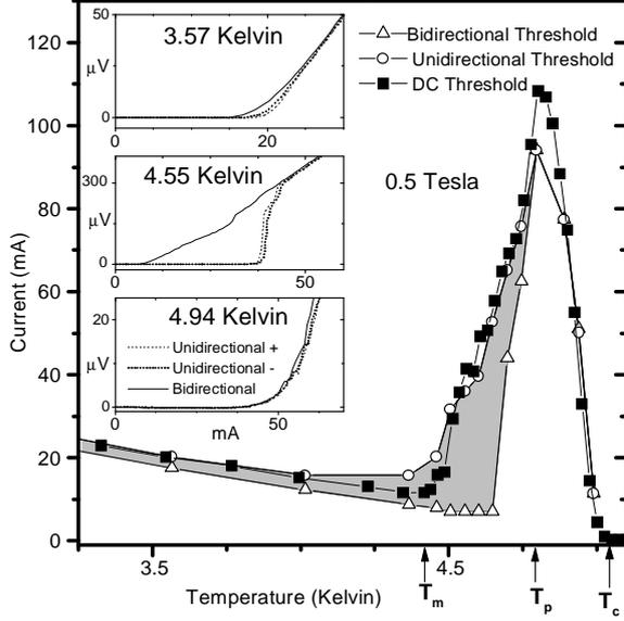
FIG. 2 Temperature dependent threshold current for unidirectional, bidirectional pulses and dc currents. Insets show the  $V$ - $I$  characteristic at three temperatures.
