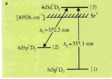
FIG. 1: A 3-level system in Strontium vapor with coupling wavelength  $\lambda_c$  and probe wavelength  $\lambda_p$ . [9]
