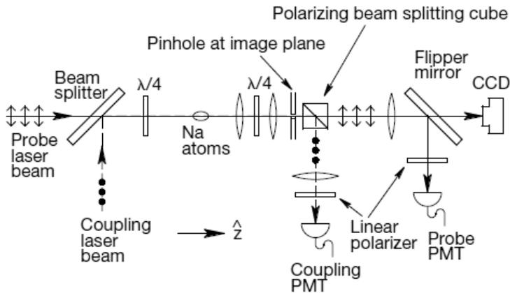
FIG. 4: An experimental set-up for EIT based optical information storage in cold sodium gas.[3]
