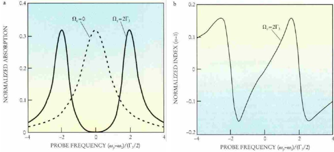
FIG. 2: a. Absorption spectrum as a function of the probe detuning with and without the coupling laser applied. b. Refractive index as a function of the probe detuning from resonance.  $\Omega_c$  is the Rabi frequency of the coupling field.  $\Gamma_3$  is the decay rate of the excited state. [9]
