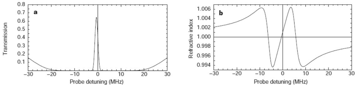
FIG. 6: a. Transmission spectrum of the probe as a function of the probe detuning from resonance in an ultracold sodium gas. b. Refractive index as a function of the probe detuning from resonance in an ultracold sodium gas [6]
