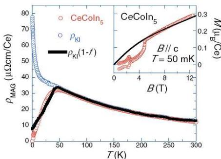
FIG. 9: Magnetic part of resistivity, defined as the difference between CeCoIn<sub>5</sub> and LaCoIn<sub>5</sub>. Red open symbols are CeCoIn<sub>5</sub> and blue open symbols are the magnetic resistivity measured in the single impurity limit. Black line is resistivity calculated by multiplying the single impurity limit data by  $(1-f)$ . Figure from [17].
