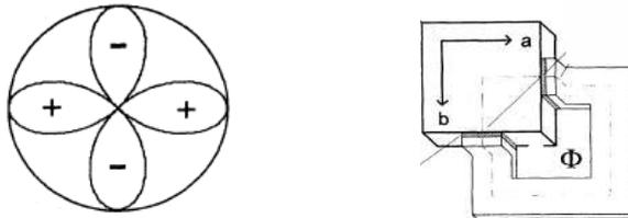
FIG. 10: Sketch of the  $d_{x^2-y^2}$  order parameter in a crystal. Drawing of a corner squid interferometer. Figures taken from [18].
