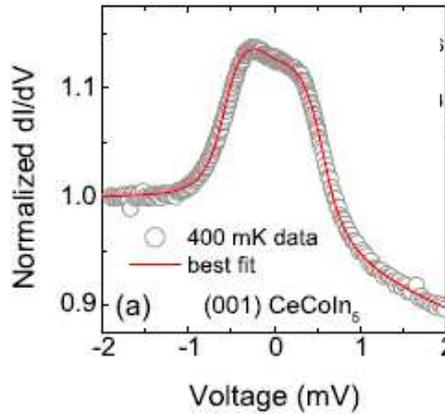
FIG. 4: Fit to data using the modified BTK model. Parameters for the curve are  $\omega_h = 0.51$ ,  $\Delta = 066\mu\text{eV}$ ,  $\Gamma = 95\mu\text{eV}$ ,  $Z_{\text{eff}}=0.28$ ,  $\eta = 1$ ,  $\Lambda = 5$  meV and  $\epsilon_0=-2.1$  meV. Figures taken from [8].
