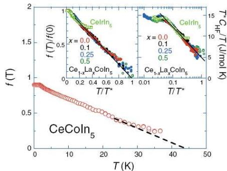
FIG. 8: The relative fraction of the heavy fermion fluid,  $f(T)$ , as a function of temperature. Dashed line is a linear fit. Figure from [17].
