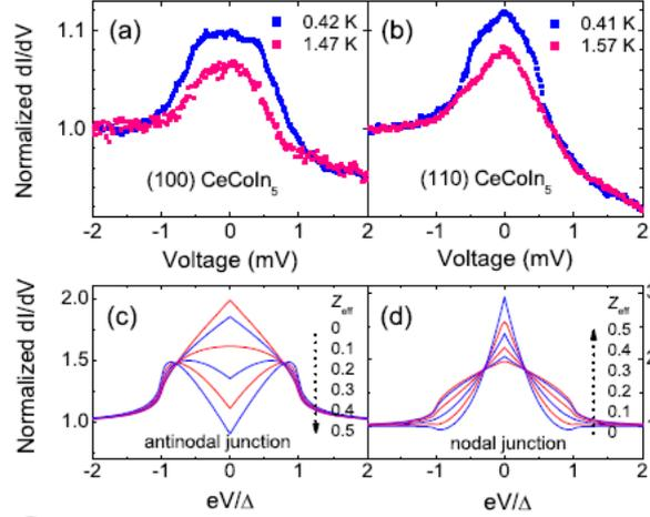
FIG. 3: Normalized conductance spectra of  $\text{CeCoIn}_5/\text{Au}$  junctions along the (a) (100) direction and (b) along the (110) direction. The data have been shifted vertically. Calculated conductance curves using the BTK model for  $d$ -wave superconductors with  $\Gamma = 0$  and  $T = 0$  for (c) antinodal and (d) nodal junctions. Figures taken from [8].
