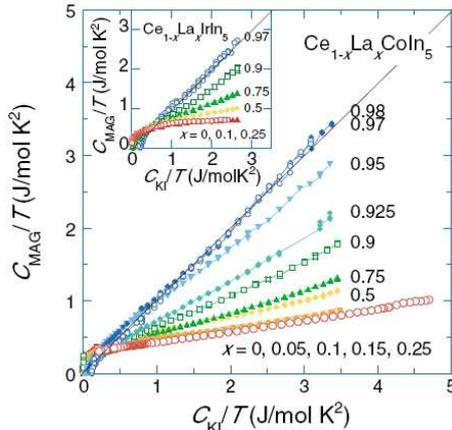
FIG. 7: The linear part of the magnetic contribution to specific heat versus the linear part of the single impurity limit. The  $x$  values given in the figure are the impurity (La) concentration from top to bottom. Figure from [17].
