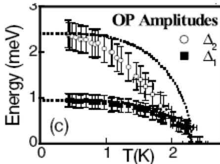
FIG. 5: Temperature dependence of the two gap amplitudes,  $\Delta_1$  and  $\Delta_2$ . At zero temperature, the gaps approach the values  $\Delta_1 = 0.95 \pm 0.15 \text{meV}$  and  $\Delta_2 = 2.4 \pm 0.3 \text{meV}$ . (figure from [4])
