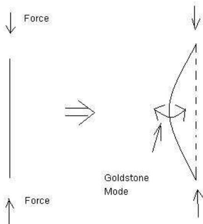
Figure 1: Compressed rod
