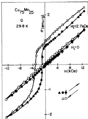
Figure 3: Magnetization,  $\sigma$ , vs. applied field,  $H$ , for quenched  $\text{Cu}_{75}\text{Mn}_{25}$  at 30 K after zero-field cooling (circles) and after  $H_c = 12.7$  kOe (triangles). Filled symbols represent data taken in ascending fields, and empty symbols represent data taken in descending fields. From reference [6]
