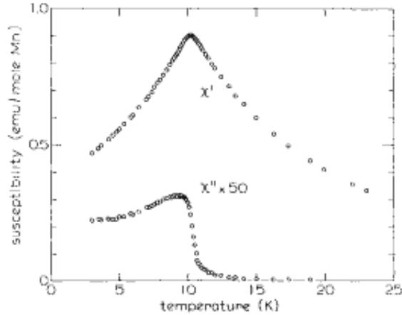
Figure 2: Temperature dependence of the susceptibility  $\chi'$  and  $\chi''$  for AuMn in zero static external field. From reference [5]
