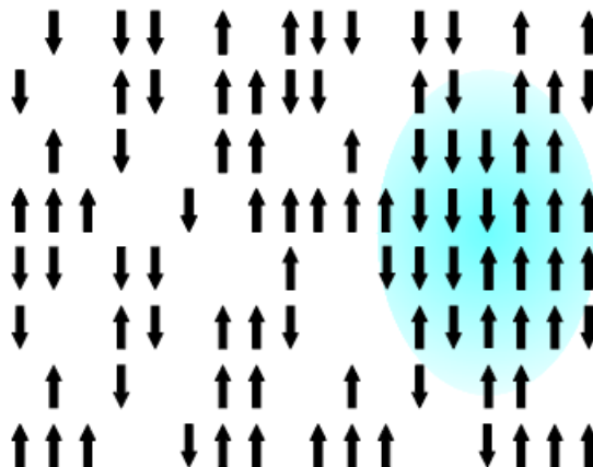
Figure 1: A randomly diluted magnet in 2d the shadowed area is the rare region, where we have an undiluted magnet. Taken from [2]. The probability of finding a large rare region decays exponentially as its volume is increased.
