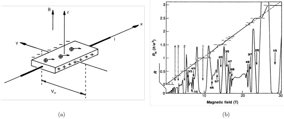
Figure 1: a) Schematic quantum Hall effect setup, which results in a conductance transverse to the direction of the field. b) Summary of several experimental signatures of the quantum Hall effect. The quantized filling fraction,  $\nu$  can be seen from the plateaus in the resistance curve
