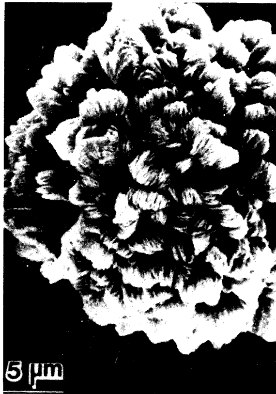
Fig. 1. Spherulite of poly-(phenylene sulfide) grown from solution, clearly showing the presence of two distinct levels of organization: a macroscopic morphology, and a microscopic, lamellar morphology. Figure by kind permission of H.D. Keith and F.J. Padden, Jr.
